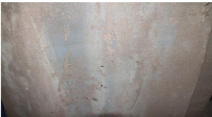
Fig.3. Geogrid sample extracted from the soil
