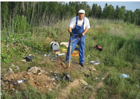
Figure 3. Probe installation into the borehole.
