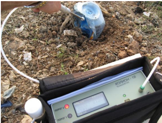
Figure 7. Air-gas environment control. Readings displayed on the monitor: TKD (metane) – 2.81%, H 2 S – 1.2%.
