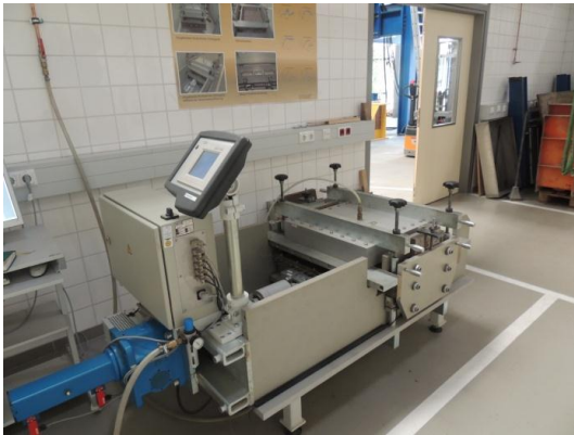
Figure 1. Apparatus for direct shear.
