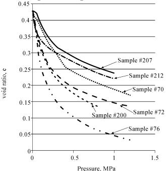
Figure 1. Compression curves for argillite samples (without water saturation)
