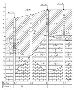
Figure 1. Geological profile of experimental construction site.
