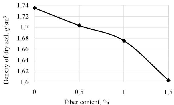
Figure 2. Dependences of dry soil density on fiber content
