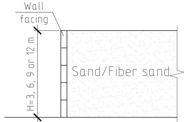
Figure 4. Design model of retaining wall.
