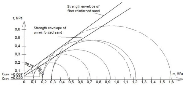
Figure 3. Mohr-Coulomb diagram for unreinforced sand and sand reinforced with 0.5% of polypropylene fiber after triaxial testing.
