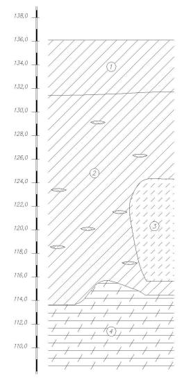
Figure 1. Experimental sites typical soil profile. Herein: 1 – soft loam and clay, 2 - soft clay and loam, with areas of gravel, 3 - loamy sand; 4 – claystone.
