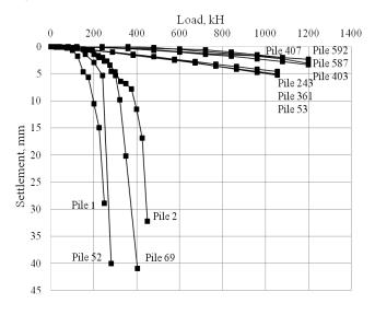
Figure 2. The pile settlement on soft clays, stiff clays and claystones  $% \left( {{{\rm{clays}}} \right)$
