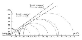
Figure 3. Mohr-Coulomb diagram for unreinforced sand and sand reinforced with 0.5% of polypropylene fiber after triaxial testing.
