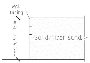
Figure 4. Design model of retaining wall.
