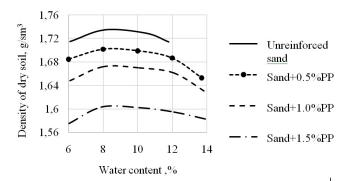
Figure 1. Dependences of dry soil density on soil water content for unreinforced and fiber reinforced sand
