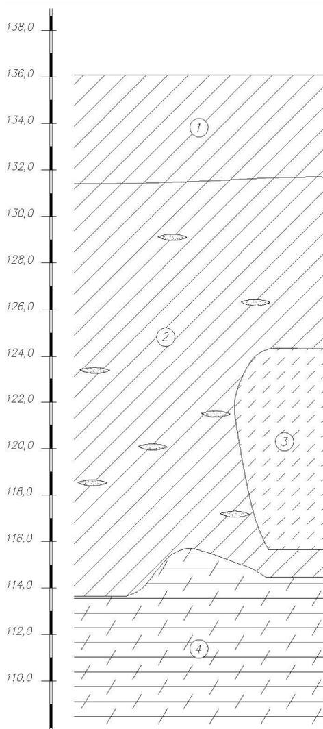
Figure 1. Experimental sites typical soil profile. Herein: 1 – soft loam and clay, 2 - soft clay and loam, with areas of gravel, 3 - loamy sand; 4 – claystone.
