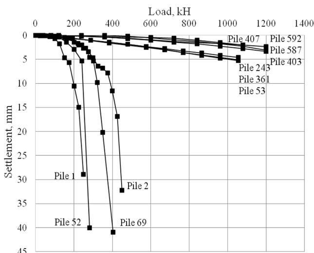
Figure 2. The pile settlement on soft clays, stiff clays and claystones
