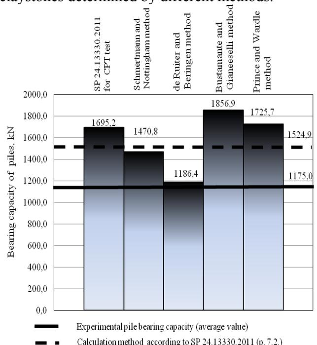
Figure 3. The average values of the calculated and experimental pile bearing capacity on claystones
